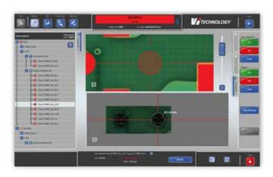
• In addition to paste inspection, PI offers simultaneous glue dot inspection.
