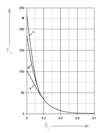
Layer thickness ≜ Material thickness: a = 1 mm b = 2 mm c = 3.6 mm
