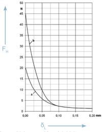
Layer thickness ≜ Material thickness: a = 1 mm b = 3 mm
