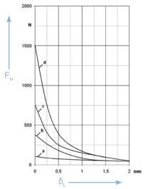
Layer thickness ≜ Material thickness: a = 1 mm b = 3 mm c = 5 mm d = 8 mm
