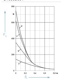
Layer thickness  $ext{\text{$\triangle$}}$  Material thickness: a = 1 mm b = 2 mm c = 4 mm d = 6 mm
